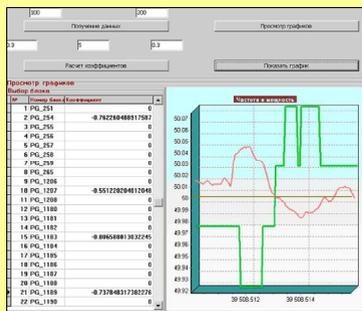
**Action of power sources in general primary regulation of the frequency in emergencies (Lab. No. 41)**
